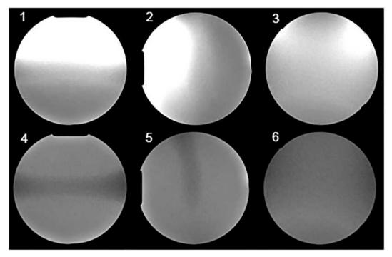
Fig. 6. Axial (1 & 4), sagittal (2 & 5) and coronal (3 & 6) MR images of a water-filled spherical PMMA phantom (Window/Level in all images: 1000/850). Top row: images acquired without the receiver coil holder; the anterior receiver coil was placed directly on the phantom. Bottom row: images acquired with the coil holder in place, resulting in a defined distance (~2 cm) between anterior coil and phantom surface.
