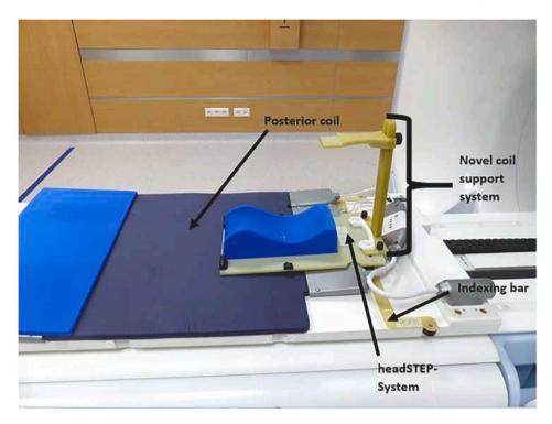
Fig. 2. Novel receive coil support system with height adjustment (set-up for head and neck tumours).
